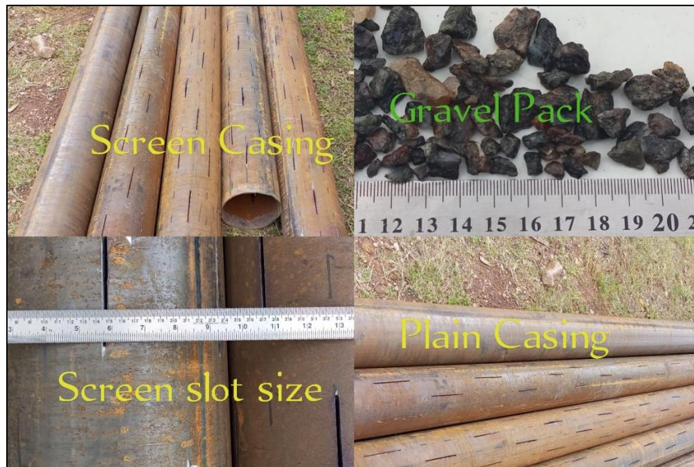
Figure 6. Casing and gravel in the two boreholes
