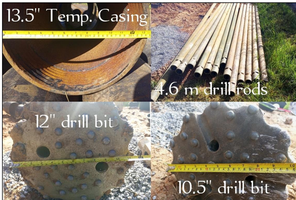
Figure 5. Drill bits, Temporary casing and rods used
