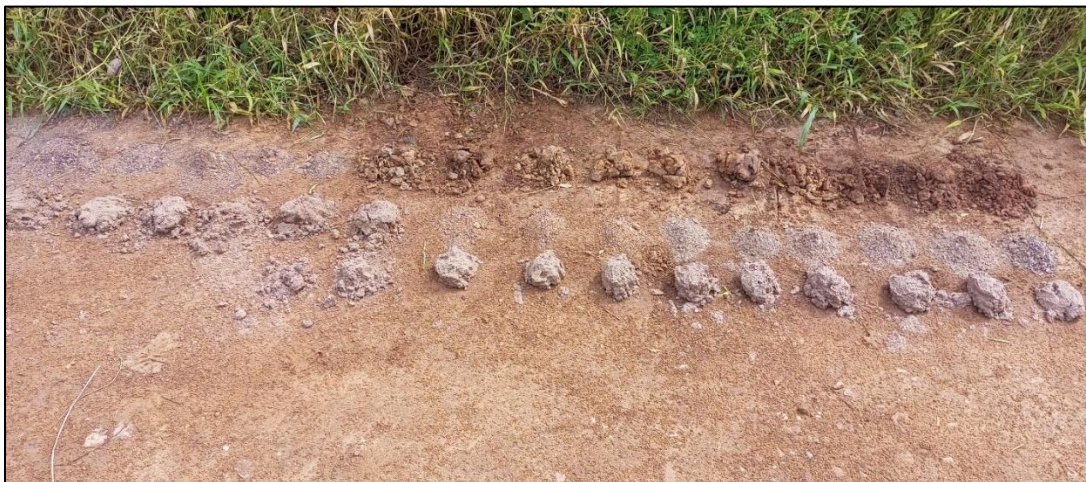
Figure 4. Drill cuttings for PH01, collected every 2 meters (0-2m at top right, 78-80m at bottom left).
