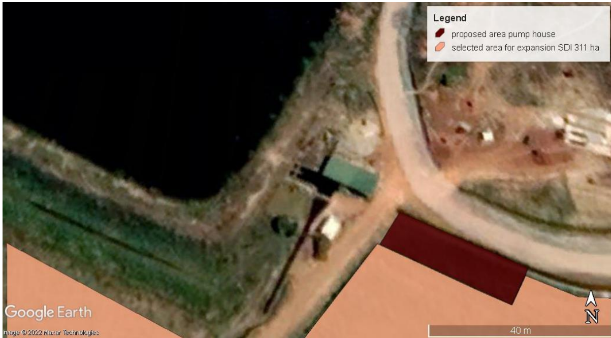
Figure 9 option location pump house though space limited, undershot gates plus canal on left side blue square will not be used anymore after installing SDI
